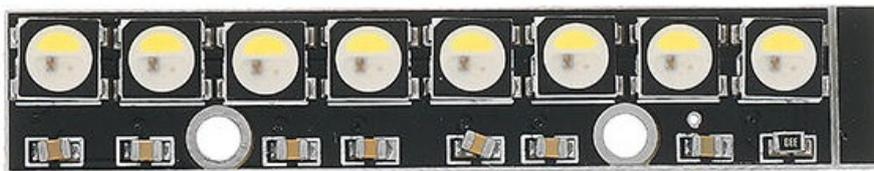
According to the specification sheet, each LED can consume 20mA at maximum brightness. That means 60mA per NeoPixel position (as there are three LEDs at each position). On my NeoPixel strip there are eight positions which will give a possible total current consumption of 480mA (assuming all NeoPixels are switched on at maximum brightness) - nearly half an Amp !!!!
