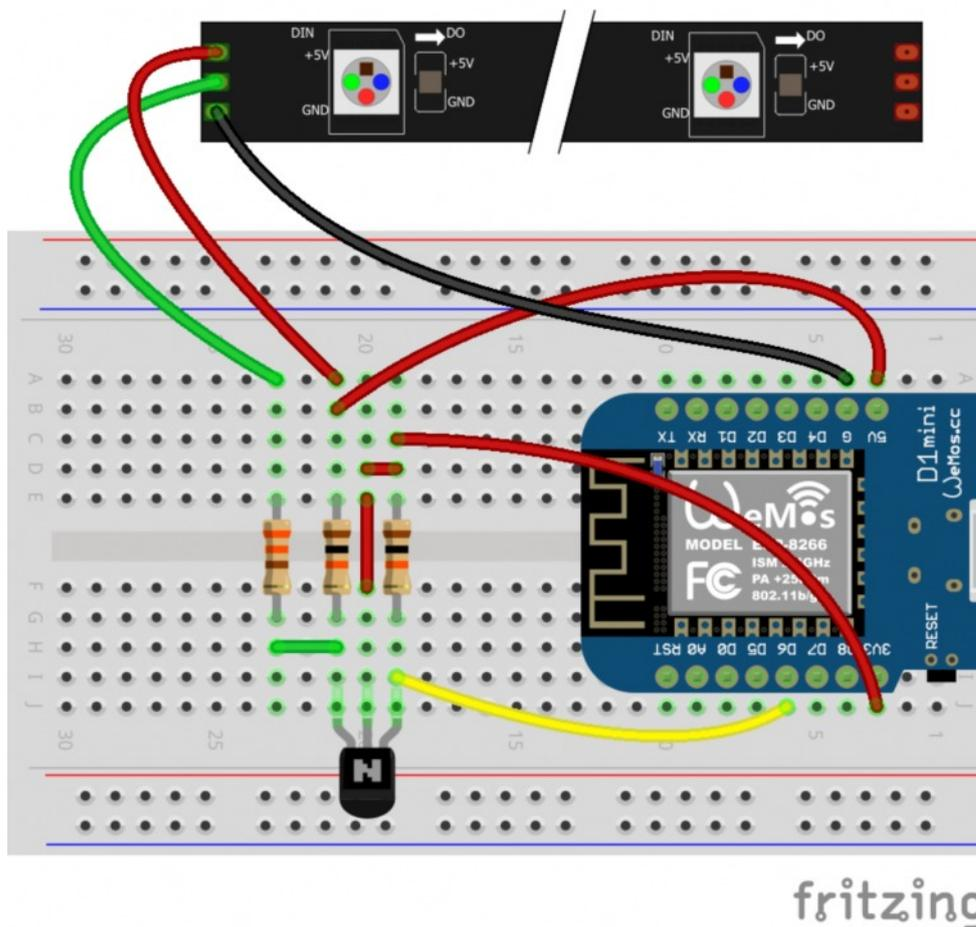
It should be noted that the NeoPixel strip needs +5V and ground. The Data-In connection uses 5V logic-levels - hence the use of the level-shifter circuit to convert +3.3V signal from the WeMos to +5V for the strip.
