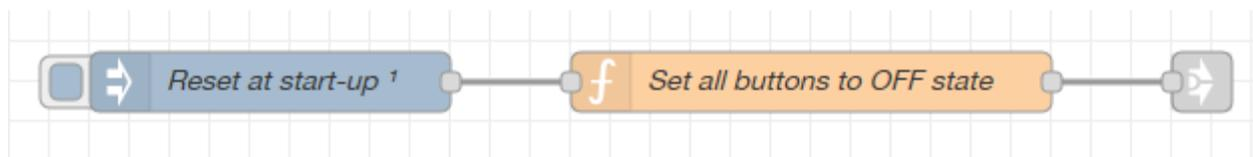
The 'inject' node labelled 'Reset at start-up' ensures the 'function' node is executed when Node-RED is started or whenever a 'full redeploy' is performed.
