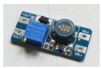
As the name suggests, it converts a lower voltage to a higher voltage. In my case it converted 3V3 (which is used to power the Wemos D1 Mini) to 12V for the IR detector. The specification says the IR detector will work off any voltage between 9V and 15V, so I thought 12V would be a good choice as it allowed a bit of
