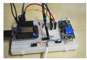
Two of the cable's cores are used to pass 12V and 0V to the unit whilst the other two connect to the voltage-free contacts.
